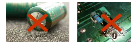
capacitor bulge and leakage
